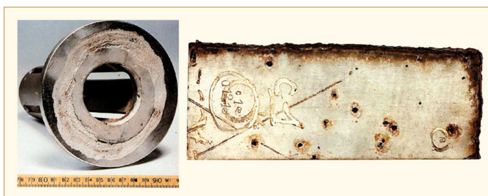
Figure 4-2: Examples of crevice corrosion damage on Type 316 stainless steels in chloride environments: left, corrosion under a gasket in brackish water, [During, 1991] - right, corrosion under deposits in a tank washed with sea water and subsequently inadequately rinsed [Désestret, 1975].
