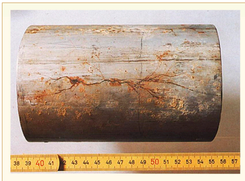
Figure 4-3: Example of stress corrosion cracking of a Type 316 stainless steel under thermal insulation at 50 to 60°C. Rinsing water containing 60 mg/kg of chloride and residual stresses are at the origin of cracking, [During, 1991].
