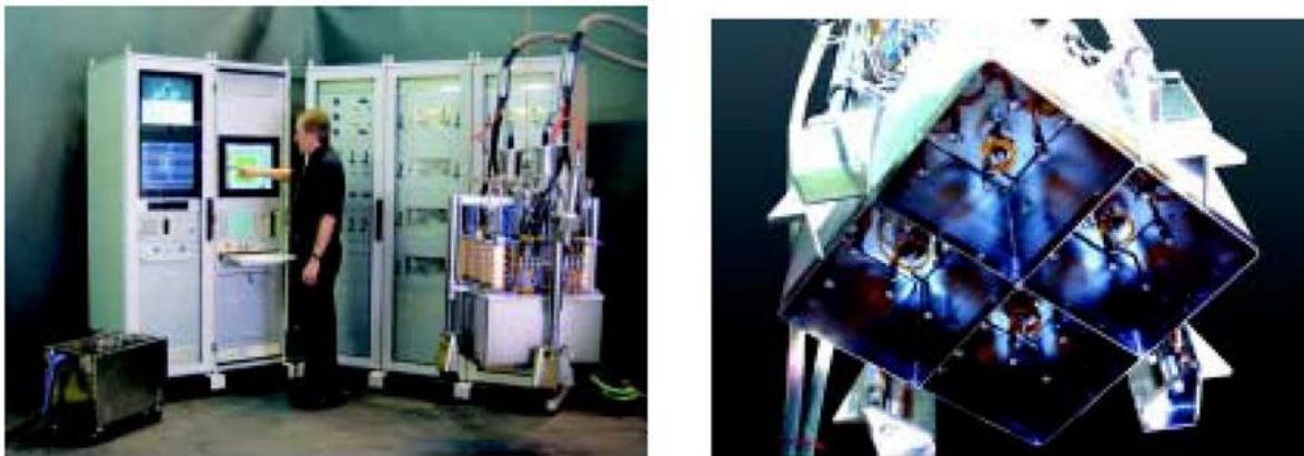
Figure 4-2: Wet in-core sipping system with control and data acquisition modules, detector and housing and 16 bundle sampling hood, modified according to [Knecht et al., 2001].
