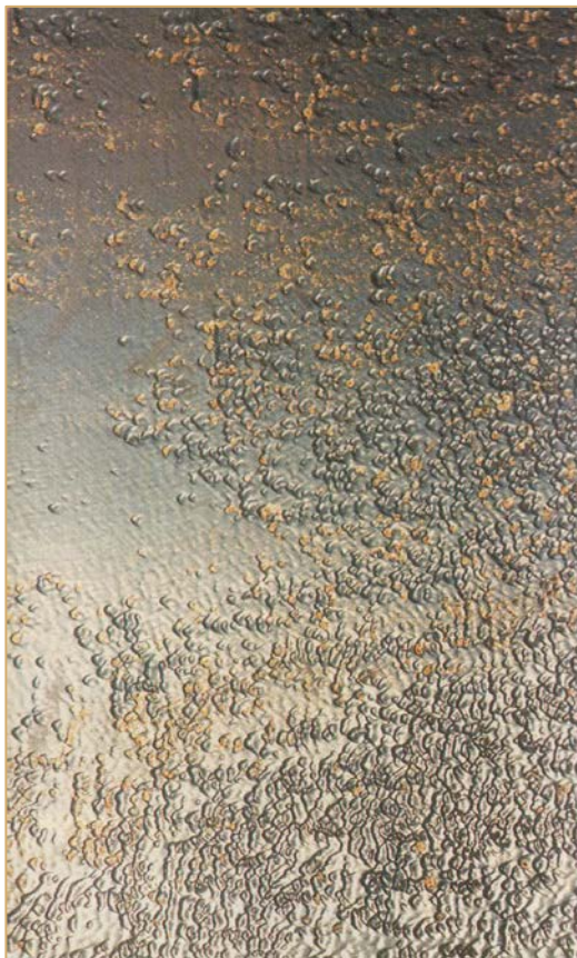
Figure A-3: The shot-peened aspect of the surface of the tube support plates results from corrosion-erosion [Mousset, 1990].
