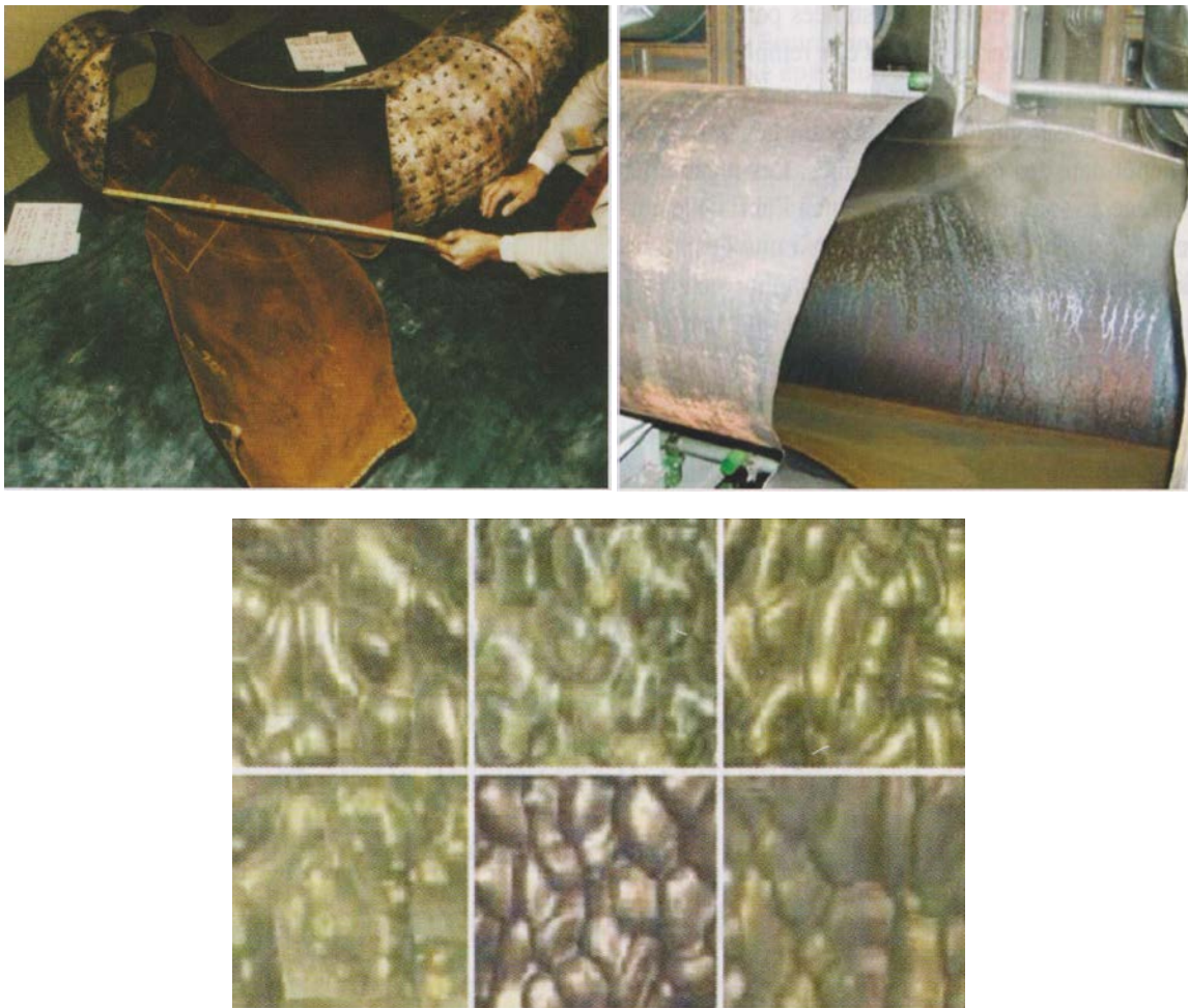
Figure 5-2: View of bursts of feedwater pipes at Surry (top left) and Mihama (top right) following flow assisted corrosion wall thinning mechanism. Bottom: typical aspect of flow assisted corrosion ID features [Hutin, 2016].
