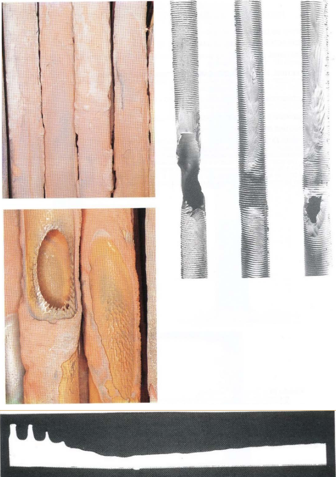
Figure B-1: Top left: iron oxides deposits covering the tubes' end. Bottom left: end of the lower tubes at the periphery showing through wall erosion. Top right: area damaged by local corrosion-erosion, then by erosion close to a tube spacer plate. Bottom: axial cut of a zone damaged by corrosion-erosion [Mousset, 1990].
