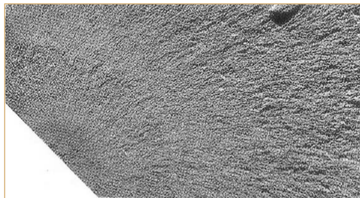
Figure D-2: Detail of the initiation zone where a dark lunula has been observed. Beyond, a first propagation zone is visible [Mousset, 1990]
