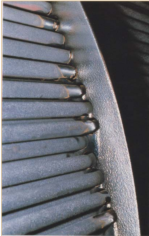
Figure A-2: View of damage to tube support plates and to tubes in the vicinity [Mousset, 1990].
