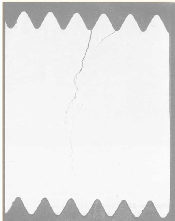
Figure H-3: Branched cracking observed on an axial section of a stud [Mousset, 1990].
