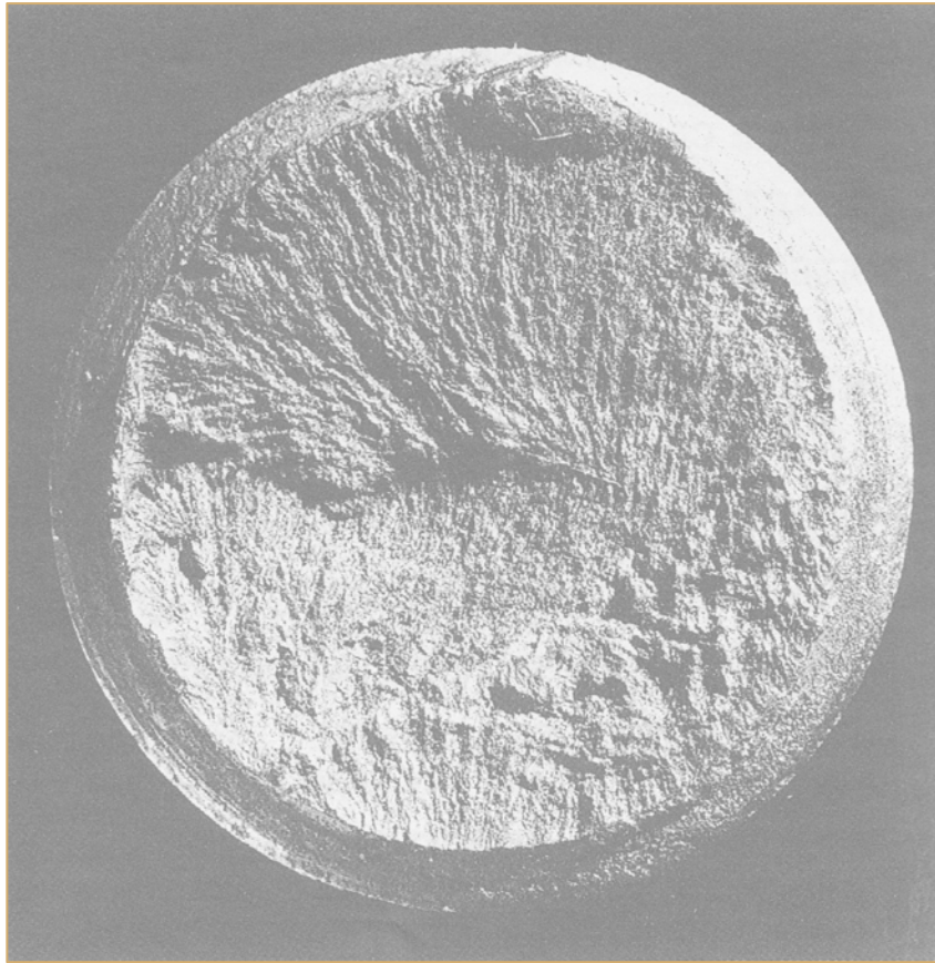
Figure H-2: Rupture by stress corrosion cracking propagating from peripheric initiation sites [Mousset, 1990].
