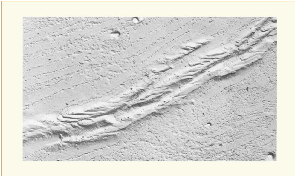
Figure 2-3: One of the earliest micrographs [Parry, 1966] showing the composite structure of a hydride cluster (transverse section of a Zr-2.5Nb pressure tube cooled under no external stress).
