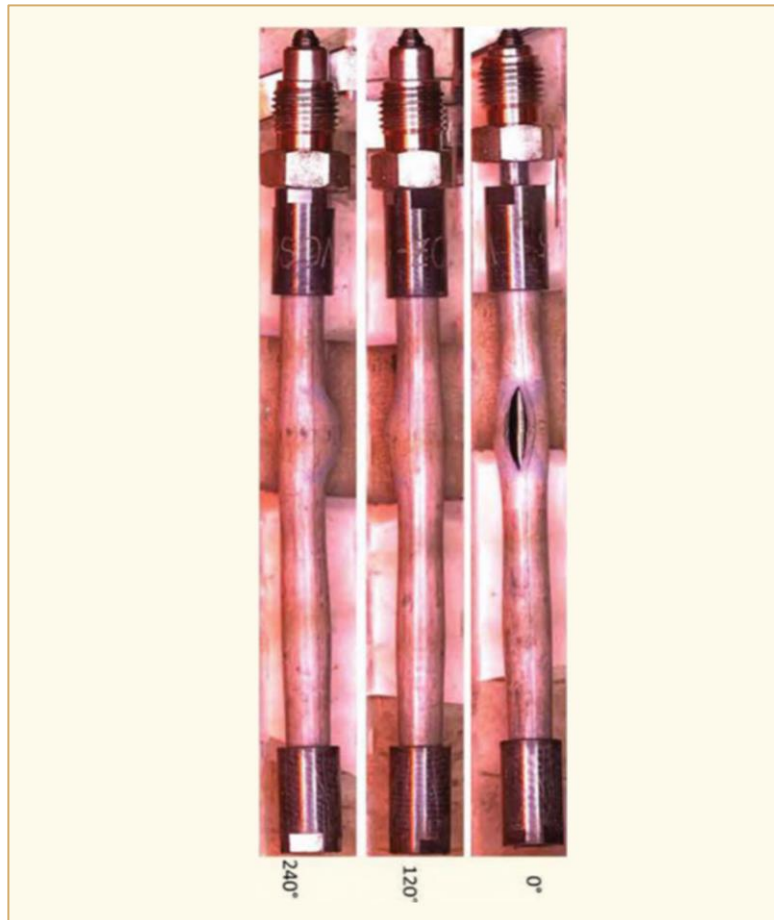
Figure 10-1: Illustration of creep rupture in cladding tubing tested to failure under constant load conditions.
