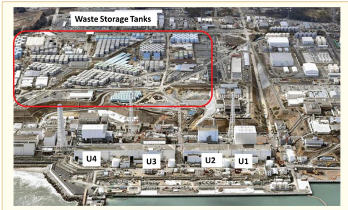
Figure 15-4: Radioactive water containing tank farm at Fukushima Daiichi Site [Reuters, 2015].
