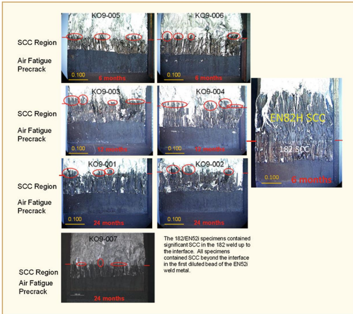
Figure 2-7: Fracture surface photographs for 182/EN52i specimens: results show a small amount of EN52i SCC extension which did not increase with additional test exposure. In contrast, significant EN82H SCC was observed after only 6 months. The scale mark is 0.1 in. (2.54 mm) [Morton et al., 2017].
