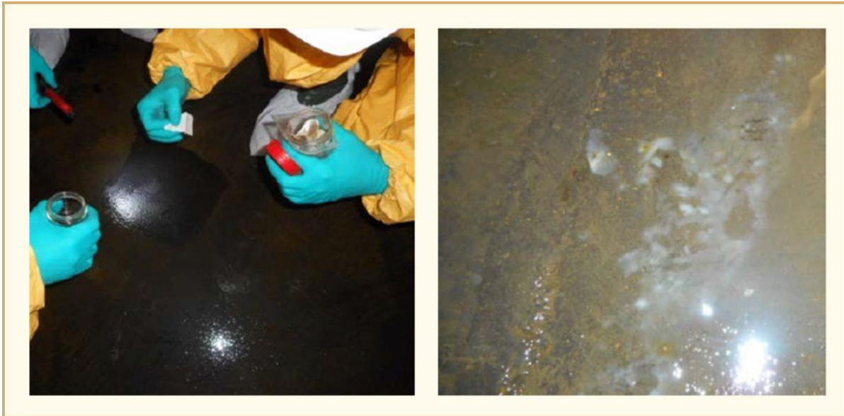
Figure 3-3: Pictures of (left) the inside of make-up tank and (right) the greasy aspect [Gressier et al., 2018].
