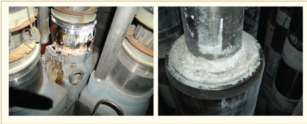
Figure 6-2: View of canopy seals leaks; left: Comanche Peak ([Baker, 2002]), right: Ringhals 4 ([Efsing et al, 2006]).
